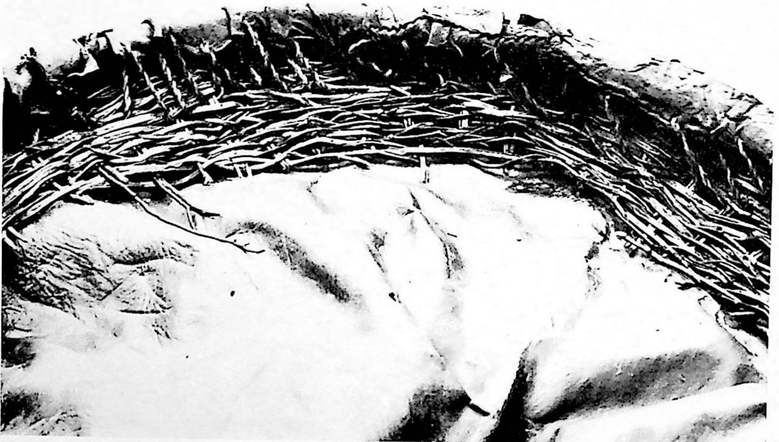
PLATE IIIb The Strathspey Currach: detail showing woven frame of rods, and horse-hair ties for the hide. Note slit in hide (on rim), sewn up with leather thongs. (Photographs: A Fenton, National Museum of Antiquities of Scotland, Nov. 1970.)
