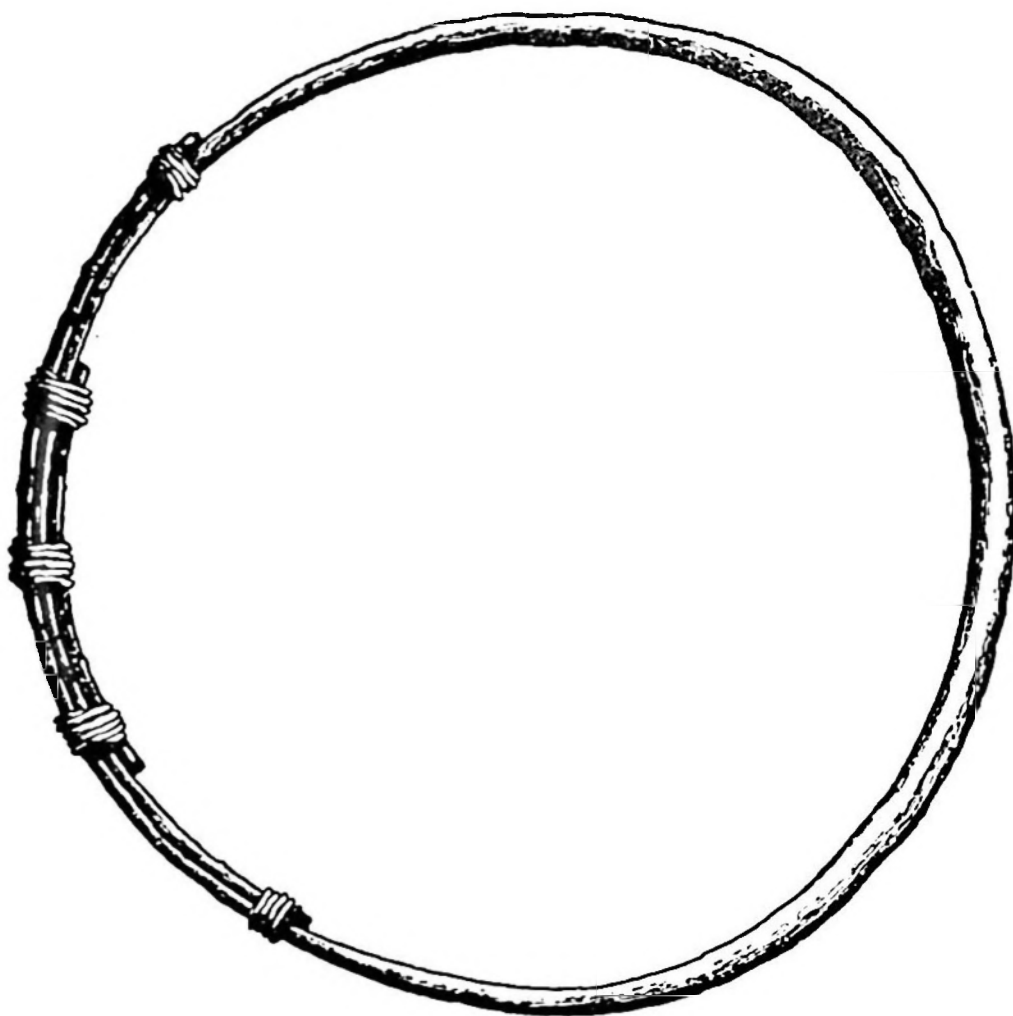
FIG. 1 The gunwale, made of a single rod whose overlapped ends are strengthened by an extra length of rod. The bindings are of withy. (Drawn by John A. Brown, 1971)
