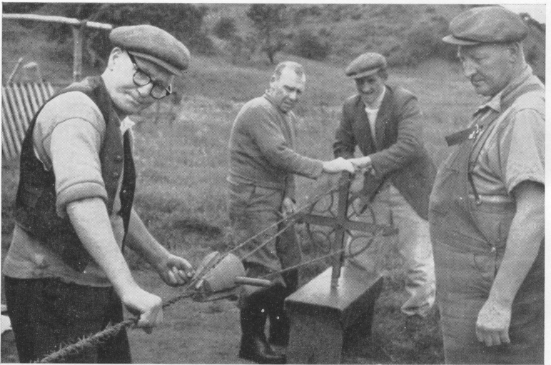
FIG. 2—Moving the tap towards the first teel, as the rope is laid (see p. 118).
